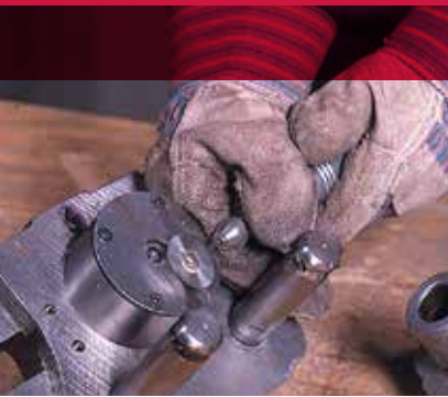
Removing galled spots from a metal forming die.
