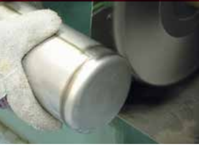
Removing heat discoloration from a stainless steel canister.
