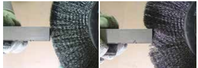
Correct Wire Tips Doing the Work
