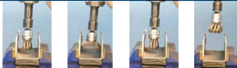
1. Insert Brush 2. Apply Power 3. Shut-Off Power 4. Remove Brush
