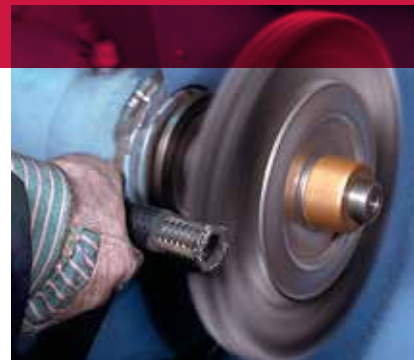
Removing rubber coating from a hydraulic hose.
