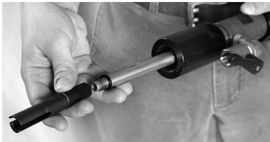
Attach coupling nut to shell cutter.
