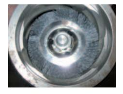
Wide face M-BRAD® wheels contain more fill material than narrow face version, providing faster cycle times and more aggressive deburring.
