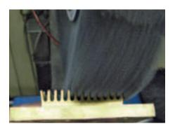
PFERD's composite wheels are for deburring, honing, edge radiusing, light cleaning, and polishing. Available with silicon carbide or ceramic oxide grain.
