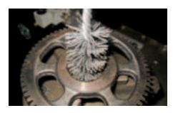
PFERD's M-BRAD® tube brushes have a non-destructive cutting action, are non-destructive to the part, and will not alter bore dimensions.
