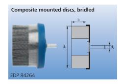
These M-BRAD® composite mounted discs are ideal for flat surfaces with holes and low projections. Especially effective on aluminum, cast iron, brass, copper and hardened steels. Bridle reduces filament flare during use. The bridle increases brush aggressiveness for applications where larger burrs need attention.
