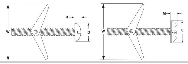
Toggle bolts are spring wing type hollow wall anchors designed for light duty use in block, gypsum wallboard, and other hollow base materials. The part is a two component assembly consisting of a machine screw and a spring wing toggle.
