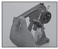
Step 7. Pull gently on Fluid Element Dispense Tube to align it with the center of the rollers.
