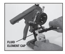
Step 4. Align **Fluid Element Cap** so it will slide into **Bottle Holder Tray.**
