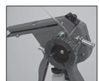
Step 5. Pull gently on Fluid Dispense Tube to align it with the center of the rollers.
