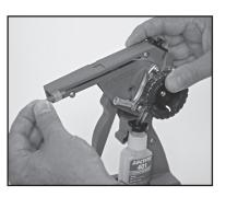
**Step 10.** Slide Vent Tube Clamp down to ensure Vent **Tube** is securely fastened.
