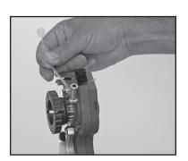
**Step 10.** Select Dispense Tip and install onto Luer Fitting. Secure fluid line into holder by pushing into groove. Insure that the tip is secure by pushing against the back wall of the holder.
