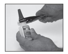
Step 7. Pull gently on Vent Tube and place into groove. Clamp in place with Vent **Tube Clamp.**
