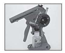
Step 6. Remove **Fluid Element Dispense Tube** from holder.
