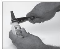
Step 3. Screw bottle into Fluid Element Cap by turning bottle. Tighten gently with pliers.
