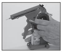
**Step 12.** Dispensing of adhesive is achieved by squeezing Trigger, touching adhesive drop onto part, and then releasing trigger.
