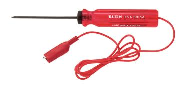
The Klein Tools Continuity Tester quickly reveals shorts or broken circuits in all types of electrical devices and controls. Tests for circuit continuity with power off. The pointed probes gets right to the problem. The handle lights up if the circuit is complete. Bulb for handle is included.
