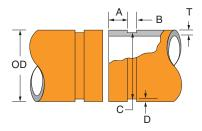
End Guard (EG) cut groove is designed for standard or heavier wall thickness pipe to be joined by HPR 7004 EG couplings. Gruvlok EG fittings are grooved in accordance with these dimensions.
