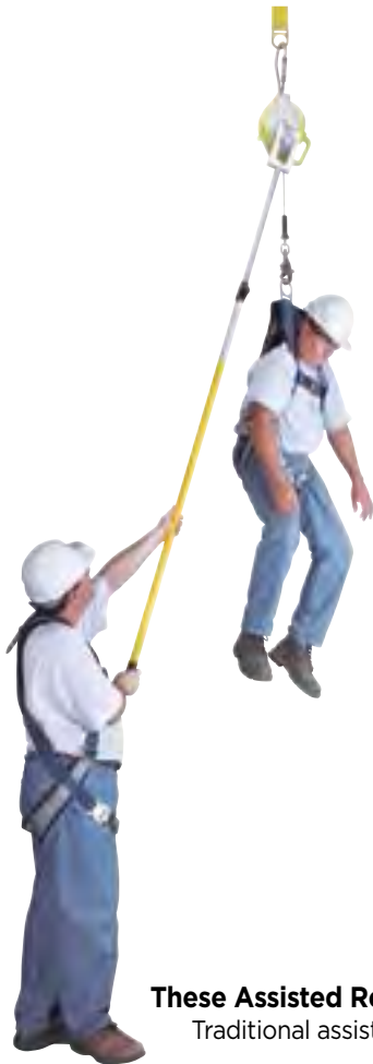
FALL ARREST MODE Assisted Rescue by Pole
