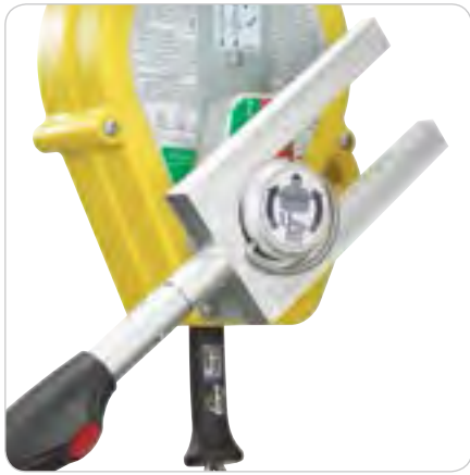
FALL ARREST MODE Assisted Rescue by Pole
